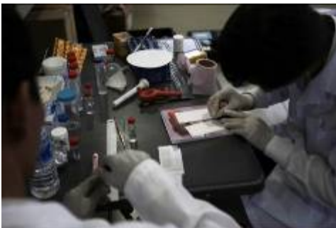
Analysts at Oddar Meanchey sentinel site test samples using thin-layer chromatography Minilab ® method
